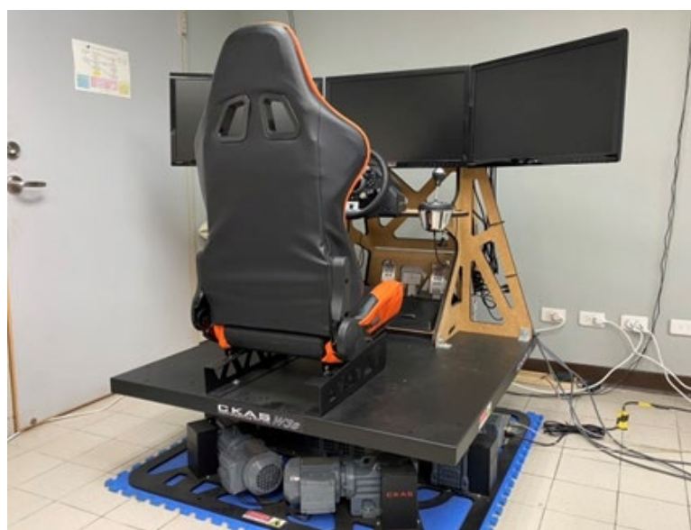
Figure 1. Driving simulator with a 6DOF motion platform.
